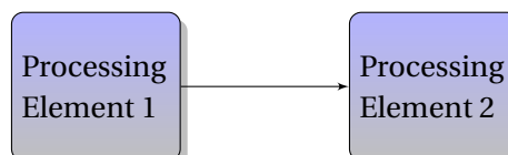
Figure 2.1: Exemplary direct connection between 2 modules
